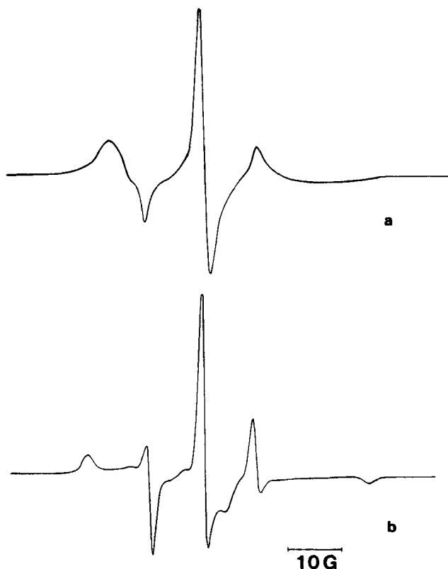
FIGURE 1 Spin label I (4.2) in random distributions of lyotropic liquid crystals at 22°C. a) Cylindrical rods b) Bilayers
